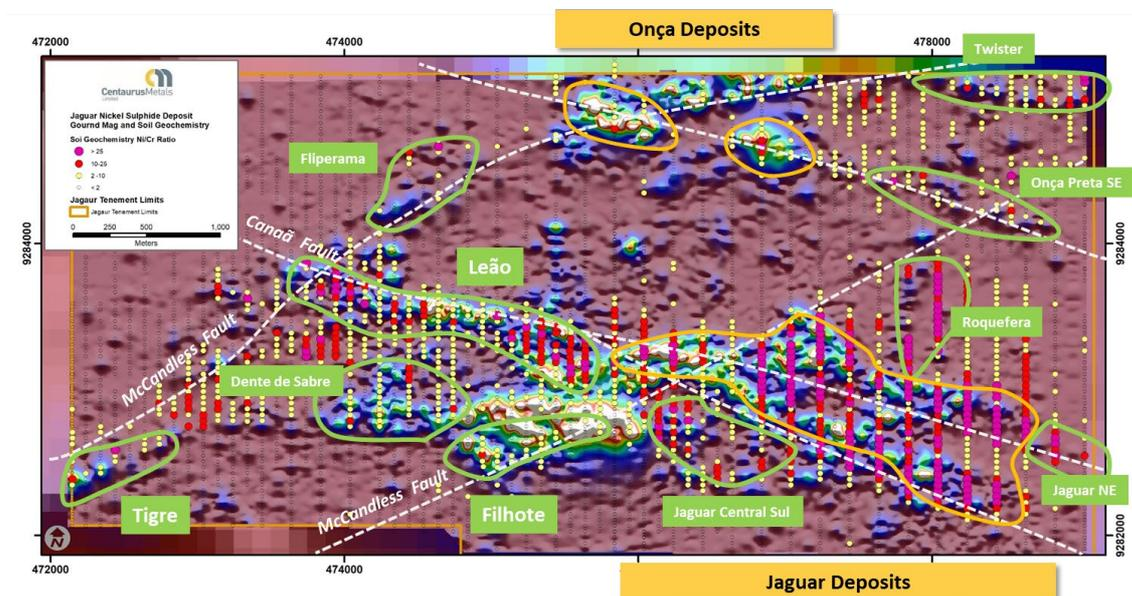
**Figure 3 – The Jaguar Nickel Project – Soils Geochemistry (Ni/Cr) over GeoTEM (Channel 12)**
