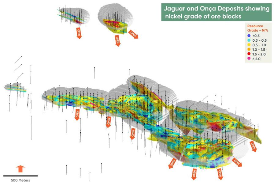
Figure 10: 3D view of the Jaguar and Onça Deposits showing nickel grade of ore blocks.
