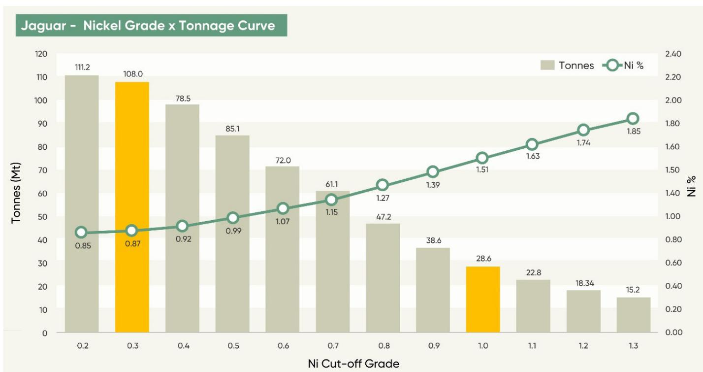
Figure 8: Jaguar Deposit – Nickel grade-tonnage curve. (Nickel cut-off grade is variable for in-pit resources but not less than 0.7% Ni for below-pit Resources).
