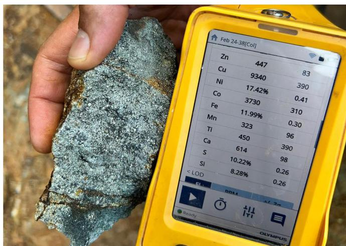
**Figure 12:** Jaguar Ore Sample – Fresh sulphides within 3 meters of surface
