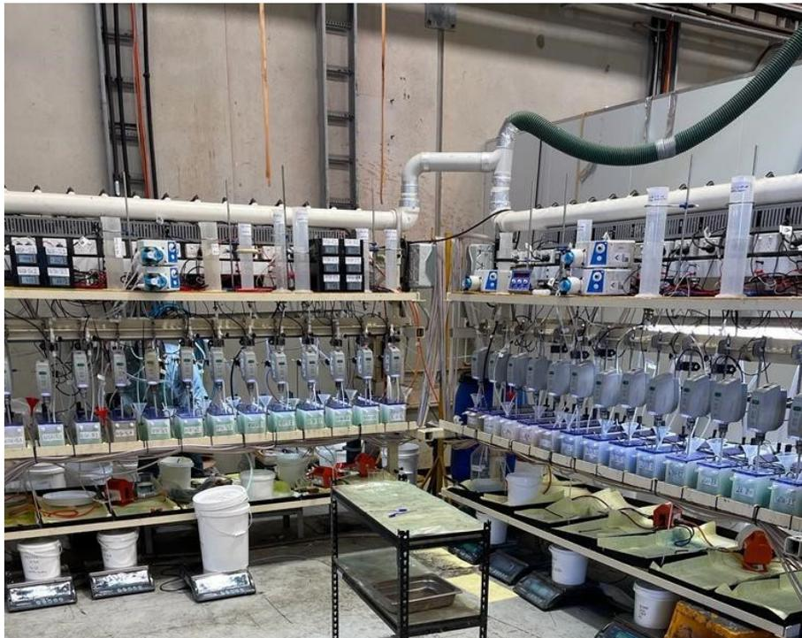
**Figure 6: Phase 3 Pilot - Cobalt and Manganese Solvent Extraction & Nickel Purification**
